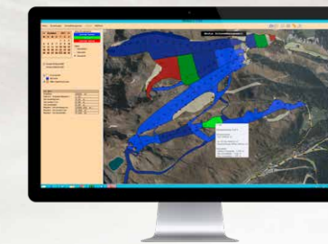
Snow management module in SNOWsat Z: The current status of the snow amount in relation to the target specification is displayed with color-coding.
