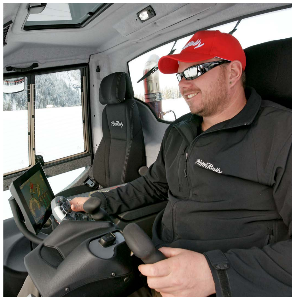
The ergonomic workstation: the intuitive joystick, the large touchscreen and the generous cockpit size make the driver's work easier.
