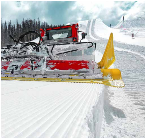
The individually folding side finishers facilitate effective work with the ParkFlexTiller.
