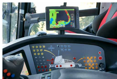
Optimised snow grooming thanks to display of routes and snow depth on the Touchscreen in the vehicle.
