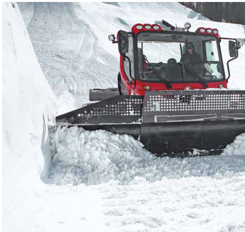
Precise cutting: the right-angled lateral cutting edge of the SwitchBlade² reduces manual work.
