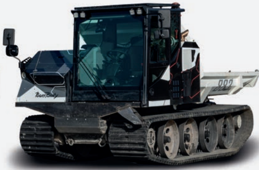
PowerBully 9D – Payload of 7.5 metric tons
