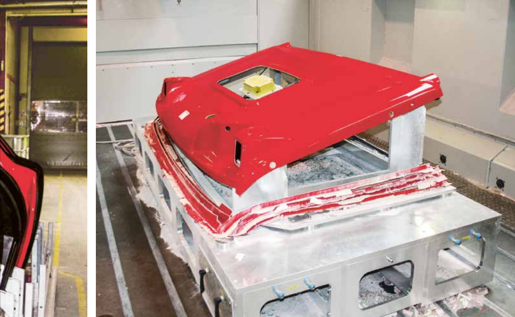
Roof of the PistenBully 600 after being machined in the new milling fixture.
