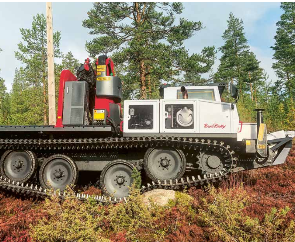
The PowerBully 18T has a payload of more than 16 metric tons. Equipped with a PK 23002 SH with gripper and basket, it is being used at a Scandinavian company. Thanks to the large dimensions of its running wheels, the PowerBully 18T adapts perfectly to the ground below it and is therefore ideal for off-road operation.
