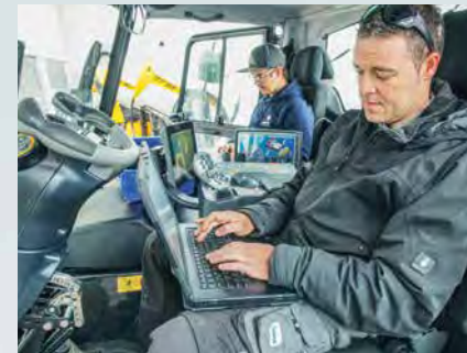
Driver's cab as test center: Together with Lorenz Schöllenger of Mattro Production GmbH, an expert on electric drives, Andreas Mayer (front) collects a wide variety of vehicle data.
