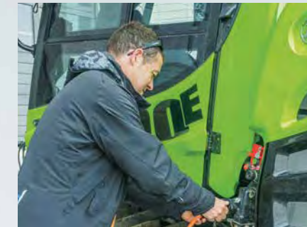
It currently takes 6.5 hours to give the battery a full charge – enough for 2.5 to 3 hours of work.
