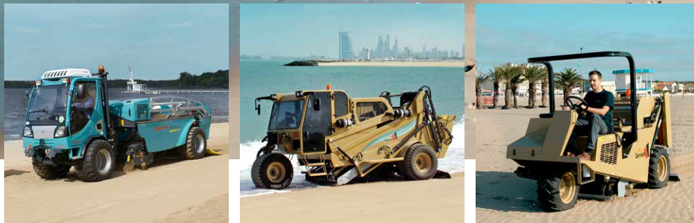
The self-propelled designs: BeachTech Marina, Cherrington 5500 and 3000 with working widths from 0.92 to 1.53 m.
