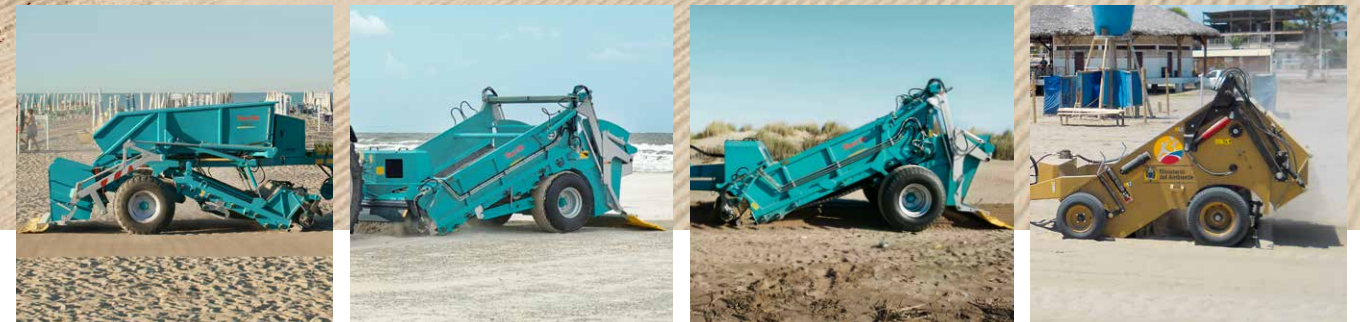
The towed BeachTech models BeachTech 3000, 2800 and 2000 are joined by the Cherrington 440 XL with working widths from 1.22 to 2.50 m.
