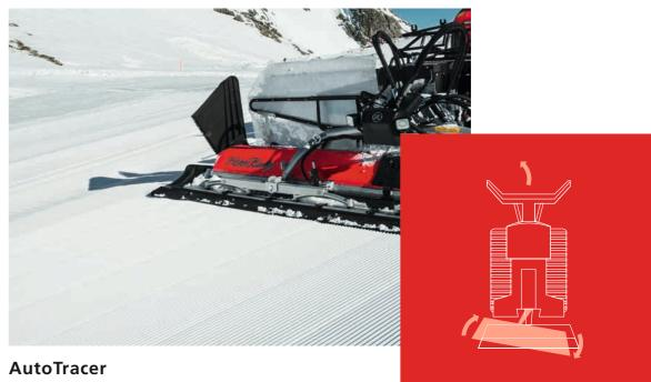
Left. Right. Left. Hands on the wheel, eyes on the slope and concentration to the max. Thanks to automatic steering support and automatic counter-steering on side slopes, AutoTracer does much of the work for the driver. Even the curviest slopes are no problem.
